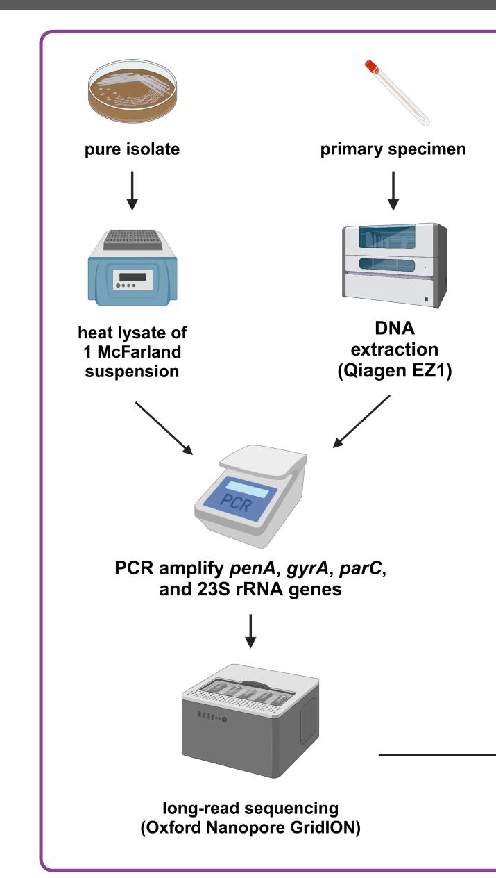
Four target genes known to be antibiotic resistance determinants are PCR-amplified from Ng DNA and sequenced on a GridION instrument (Oxford Nanopore Technologies).
