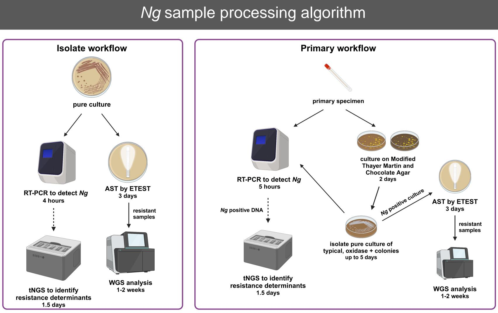
The current Wadsworth Center algorithm requires a live, pure culture of Ng to determine antibiotic susceptibility. WC frequently receives primary specimens which are positive for Ng DNA by real-time PCR, but are non-viable in culture, precluding any further characterization.
